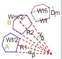
For Block A the dimesion  $R_1$  is perpendicular (has a 90 degree angle) to dimension  $W_f/2$
